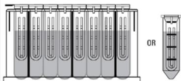
4. Place device into the deep-well plate or 2mL microcentrifuge tube containing buffer.
